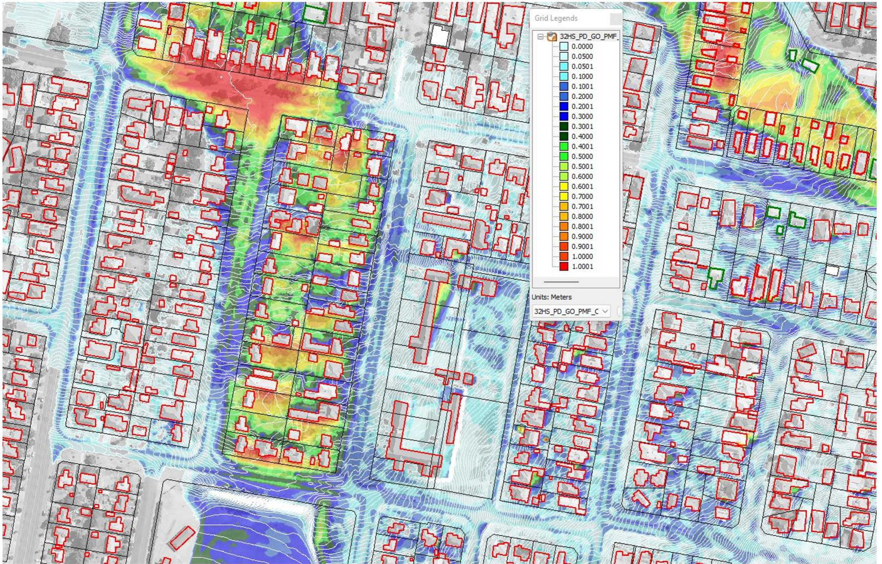
PMF TUFLOW MODEL RESULTS – PRE-DEVELOPMENT CONDITIONS [Colour legend refers to depth of inundation in metres]
