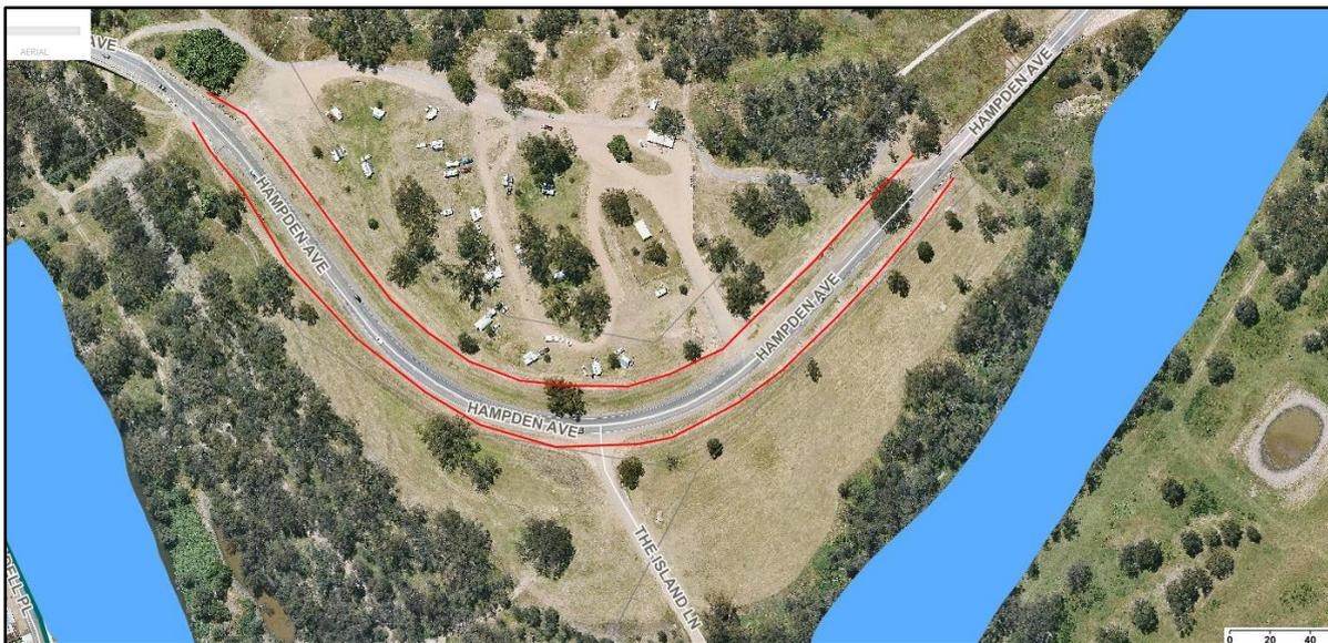
If the existing banks along Wilks Park are formalised as part of the levee construction, the section of North Wagga protected by the ring levee will be able to evacuate at more appropriate height of approximately 9.7m or 9.8m while the section of North Wagga along East Street will need to evacuate at approximately around 9.3m.
