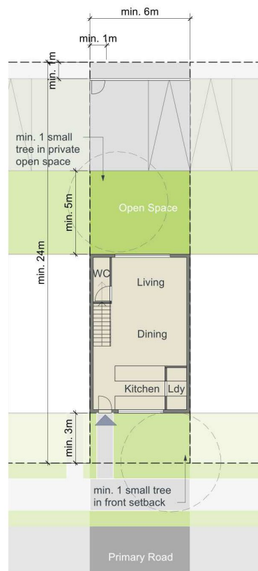
Figure 13 Rear-loaded townhouse plan
