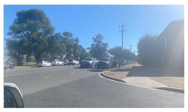
According to Austroads Guide to Road Design – Part 4A, a Safe Intersection Sight Distance (SISD) of 97 metres is required for a 50 km/h zone to allow safe decision-making for entering traffic.
