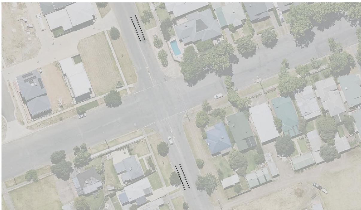
Figure 1 – Advance Warning Linemarking installed September 2026
