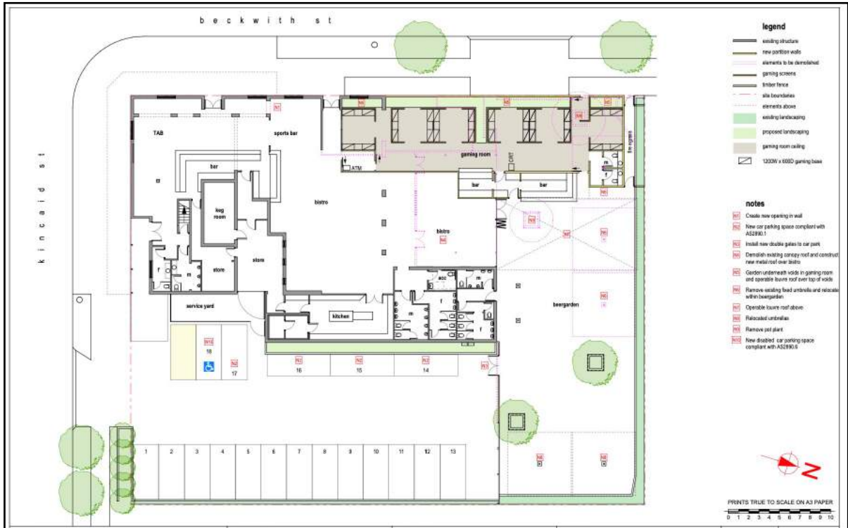
Figure 26: Proposed Ground Floor alterations & additions 2023 (Source: DMD 2023)
