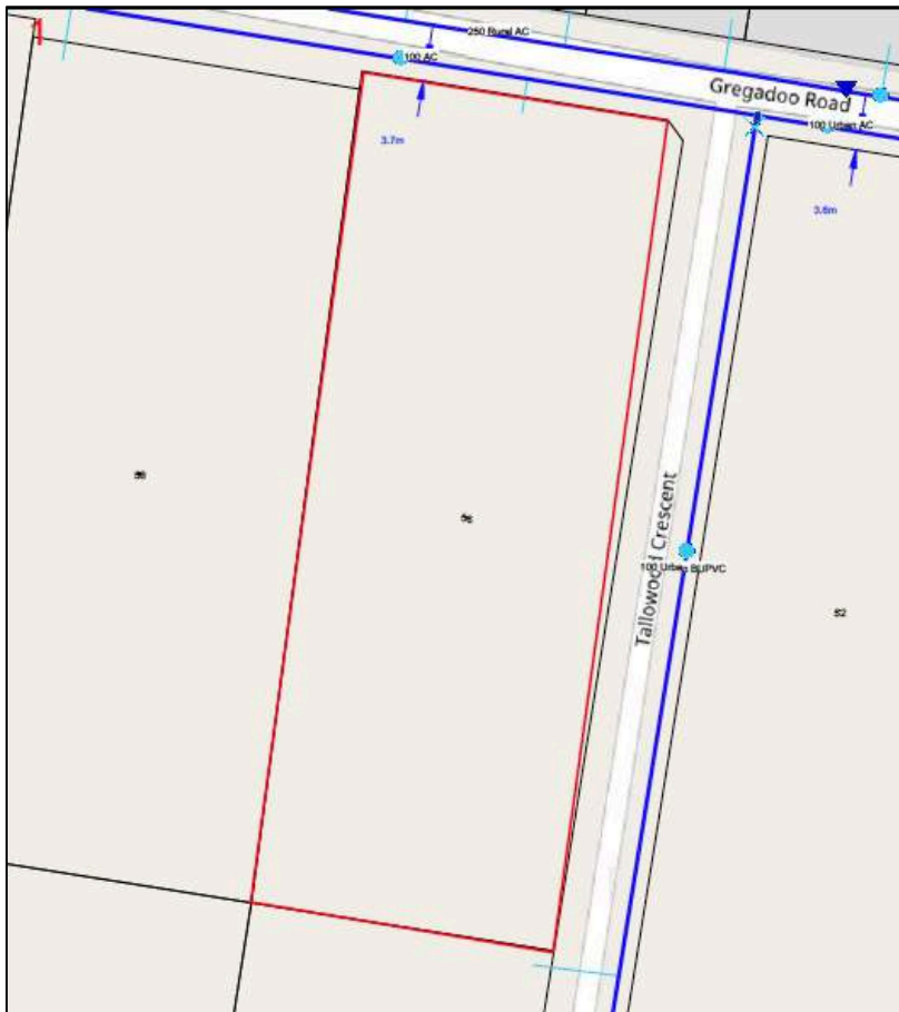
Figure A1-33: Existing Water Supply Network (Source: RWCC 2017)
