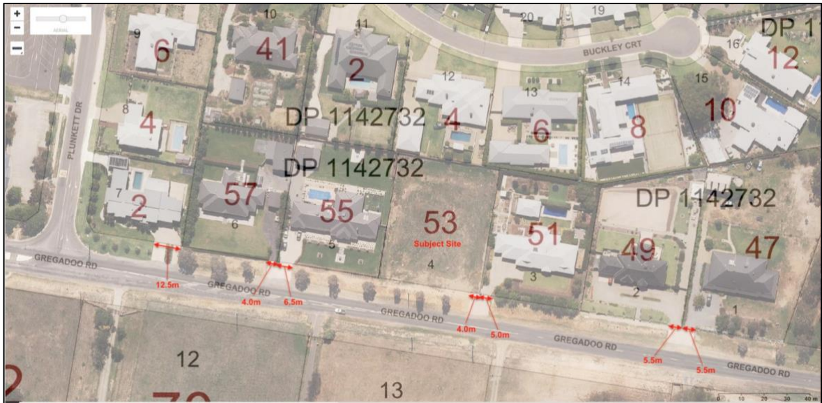
Figure 1: Driveway width analysis from common boundaries on Gregadoo Road (WWCCGIS 2021).
